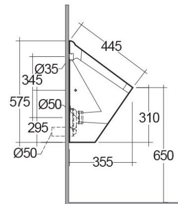
Dimensions: All dimensions in mm tolerance +/- 5% for below 200mm and +/- 3% for above 200mm.
