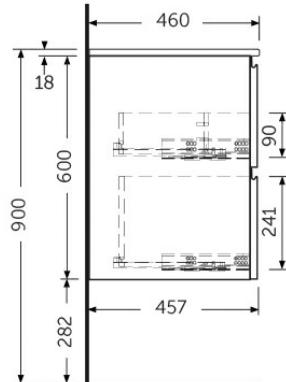
Dimensions: All dimensions in mm tolerance  $\pm 5\%$  for below 200mm and  $\pm 3\%$  for above 200mm.
