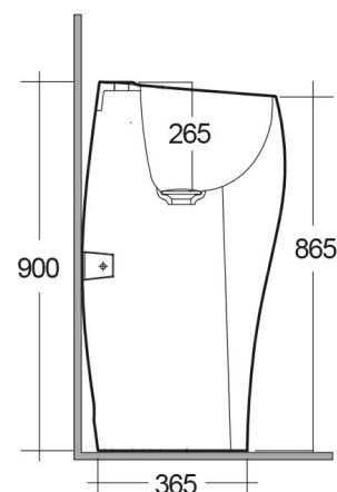
Dimensions: All dimensions in mm tolerance  $\pm 5\%$  for below 200mm and  $\pm 3\%$  for above 200mm.
