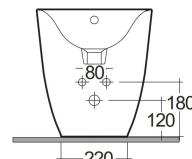
Dimensions: All dimensions in mm. Tolerance of vitreous china & fireclay items:  $\pm 5\%$  for below 200mm and  $\pm 3\%$  for above 200mm; for all other items tolerance  $\pm 1\%$ . Note: Due to a continuing development program to improve design and performance, the manufacturer reserves all rights to vary specifications without prior information. Please note accessories are for photographic use only.
