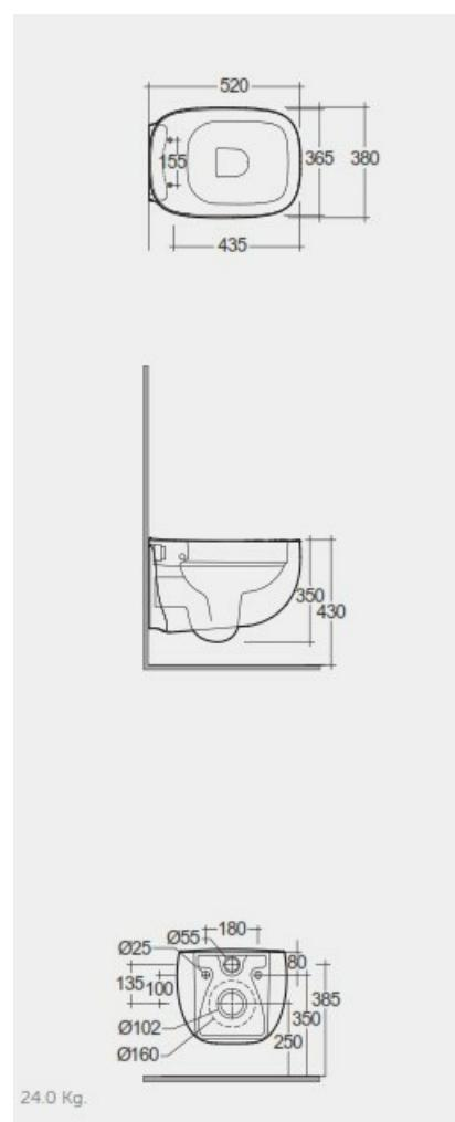
Dimensions: All dimensions in mm tolerance  $\pm 5\%$  for below 200mm and  $\pm 3\%$  for above 200mm.
