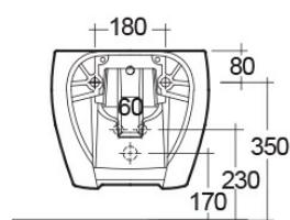
Dimensions: All dimensions in mm tolerance  $\pm 5\%$  for below 200mm and  $\pm 3\%$  for above 200mm.
