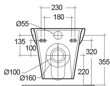
Dimensions: All dimensions in mm tolerance +/- 5% for below 200mm and +/- 3% for above 200mm.
