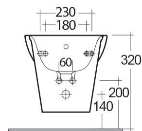
Dimensions: All dimensions in mm tolerance +/- 5% for below 200mm and +/- 3% for above 200mm.
