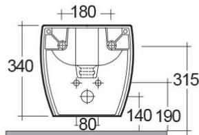
Dimensions: All dimensions in mm tolerance +/- 5% for below 200mm and +/- 3% for above 200mm.
